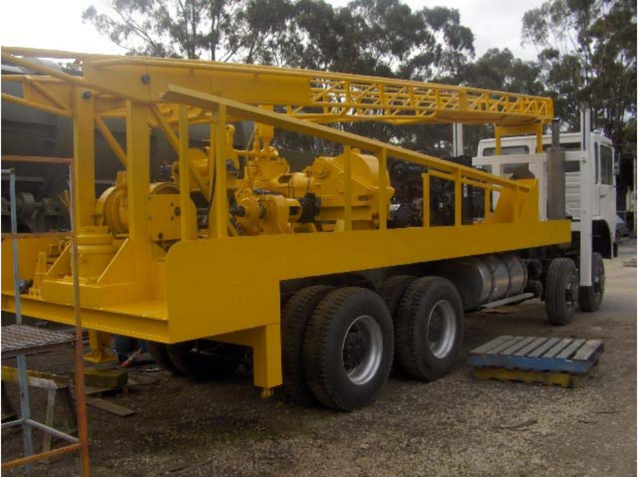
Curnamona Energy's recently refurbished 8 wheel drive drilling rig
