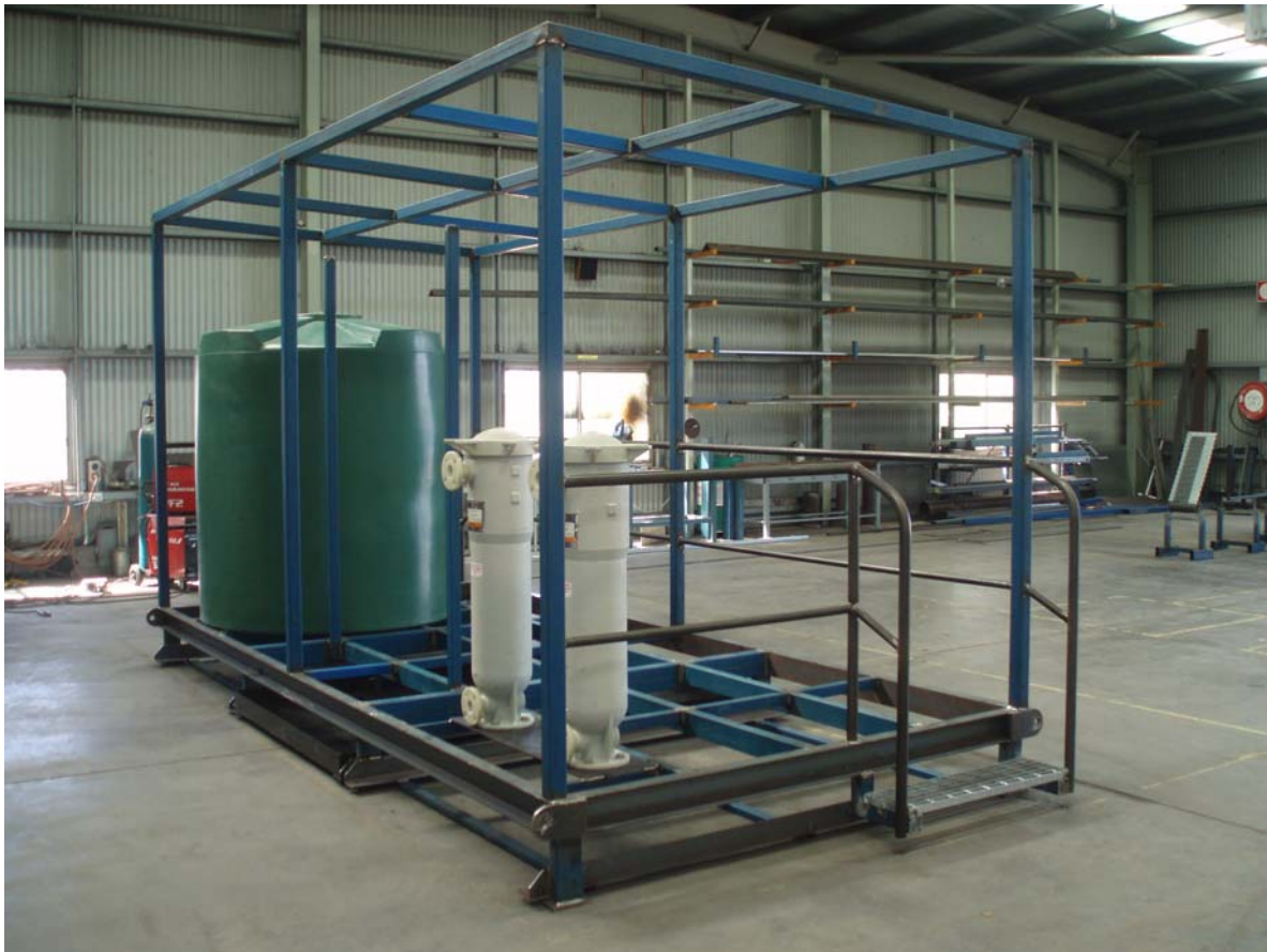
Well house in process of being fabricated by Complete Pipe Systems in their factory at Murray Bridge.
