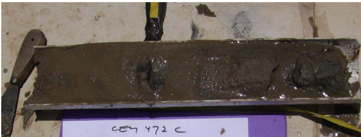
Uranium mineralized pyritic sand in drillcore from Oban. The dark colour is mainly due to pyrite and organic matter in the sands. This interval assays 830 ppm U_3O_8 .
