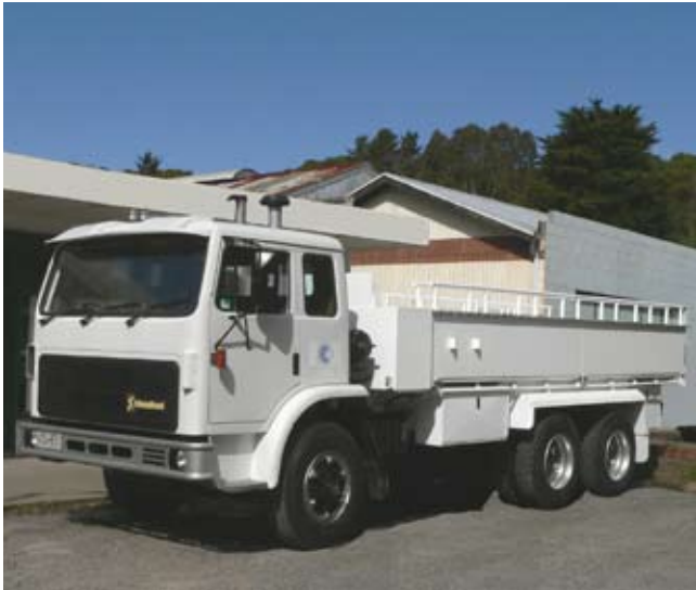
Curnamona's recently delivered water tanker, required to supply water for mud drilling operations
