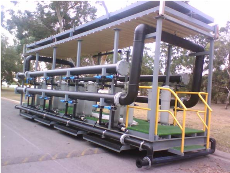
Figure 2 : Example of fabrication by Complete Pipe Systems. The well house being constructed for Curnamona Energy will be of similar design to this, incorporating a steel skid for portability and drip trays to prevent spillage.
